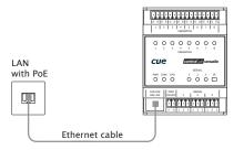
The integrated IEEE 802.3af PoE support allows installation in areas where PoE network infrastructure is installed.
