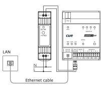
Delivered DIN rail power supply 24 VDC can be used for areas without PoF infrastructure.
