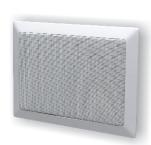
The APart CMR20T is a compact 2-way rectangular built-in speaker. It can be used as a 16 Ohm or 100 Volt loudspeaker. In 16 Ohm use, you can connect up to 4 loudspeakers in parallel on each channel of a standard 4 Ohm amplifier. For 100 Volt use, the CMR20T is equipped with a High Quality 20 watt 100 Volt transformer with several power tappings. These tappings can be selected via a switch that is hidden behind the loudspeaker grill.
